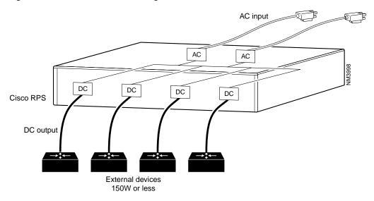
Figure 7 Fully Redundant Configuration
